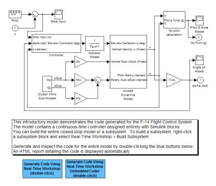
The model simulates the pilot's stick input with a square wave having a frequency of 0.5 radians per second and an amplitude of  $\pm 1$ . The system outputs are the aircraft angle of attack and the G forces experienced by the pilot. The input and output signals are visually monitored by Scope blocks.
